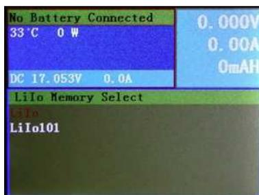
Press **ENTER/START** button for 3 seconds Edit, Add or Delete recorded memory data as right picture. one memory data has a memory name and include a set of charge and discharge parameters, you can save a set of parameters for your each battery, the charger can save up to 10 set of parameters for each battery type.
