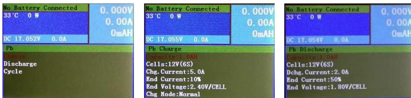
The details of parameters set up for **Pb acid battery (VRLA)** is in the following table.
