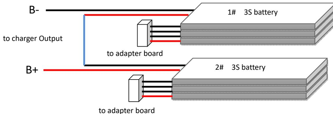
2. Plug 1# battery and 2# battery into adapter board, if plug into mistaken socket, the red LED will be on, please do it again.
