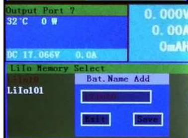
if need add new data record, first press Add and press **UP/DOWN** rename a memory name (press **STOP/SET** back to last name), then press Save and save it. after you choose new memory name and modify some parameters, the charger will record the latest parameters. Press Exit don't save any change. see right picture.
