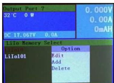
Press **UP/DOWN** alternate Edit, Add or Delete, Press Edit and **UP/DOWN** modify saved memory name. Press Delete delete saved memory data. Press Add save new data.
