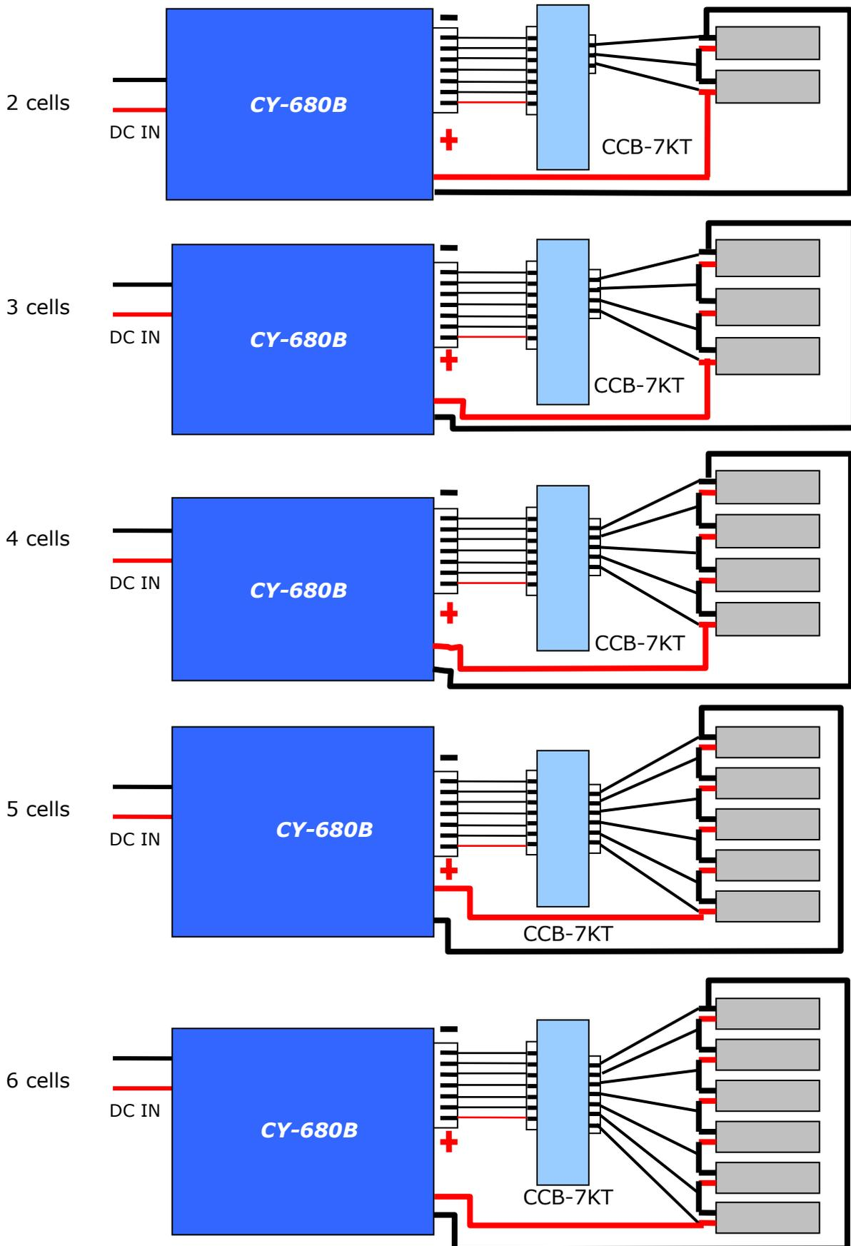
**Balance Charge 2\*5S battery packs, Please note the batteries being charged should all have the same nominal capacity (mAh).**
