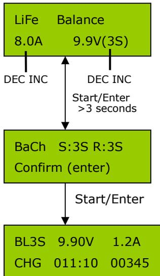
The value on the second line sets a charge current and the voltage of the battery pack. Press the **START/ENTER** button, and then press the **DEC or INC** to set value. After setting the current and voltage press **START/ENTER** button for more than 3 seconds to start the process. (Charge current: 0.1~8.0A, Voltage: 1~6 series)
