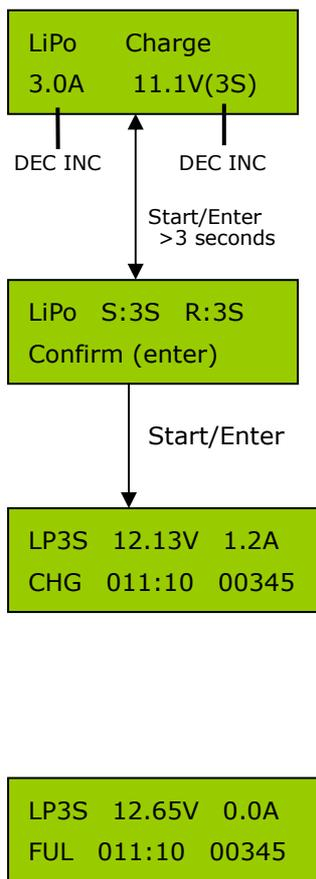
The value on the second line sets a charge current and the voltage of the battery pack. Press the **START/ENTER** button, and then press the **DEC or INC** to set value. After setting the current and voltage press **START/ENTER** button for more than 3 seconds to start the process. (Charge current: 0.1~8.0A, Voltage: 1~6 series)
